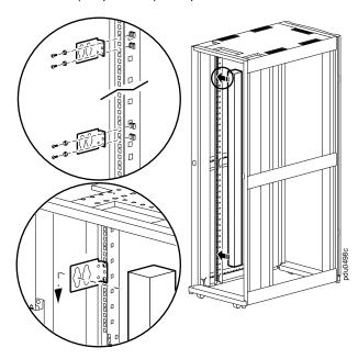
Route the power cable out of the rack and connect it to an appropriately rated branch circuit of your power source. The Rack PDU should be connected to a dedicated branch circuit protected by an appropriately sized circuit breaker. Turn the power feed circuit breaker on only after connection to the Rack PDU is complete.
