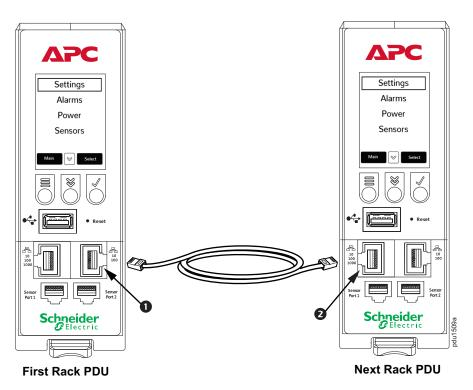
Up to 32 Rack PDUs of the same SKU can be connected using a single IP address. The Rack PDUs are cascaded from the first Rack PDU to the next.
